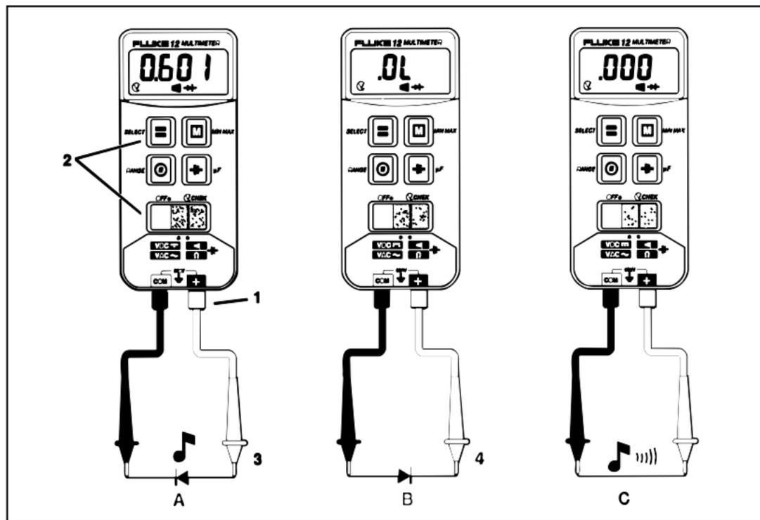
Figure 5. Testing Diodes
